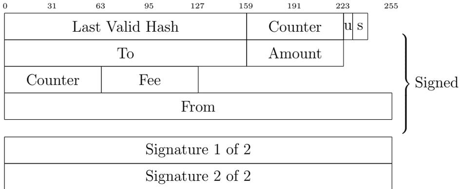
With payload the minimum size: 176 bytes
