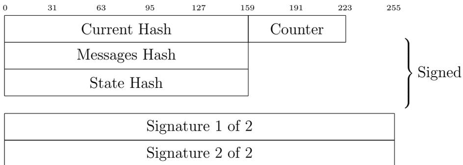
Minimum size of the output packet is: 132 bytes
