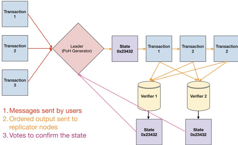
Figure 1: Transaction flow throughout the network.
